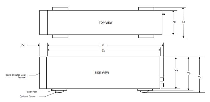
Figure 1. Dell EMC PowerEdge T440 system dimensions
