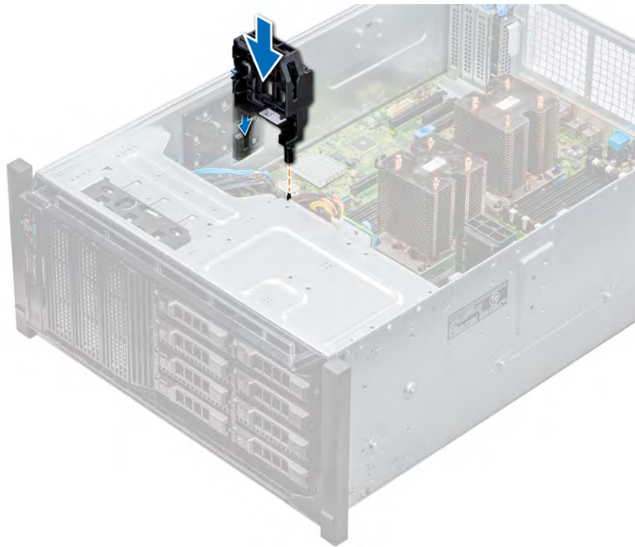
Figure 76. Installing the optional GPU card holder
