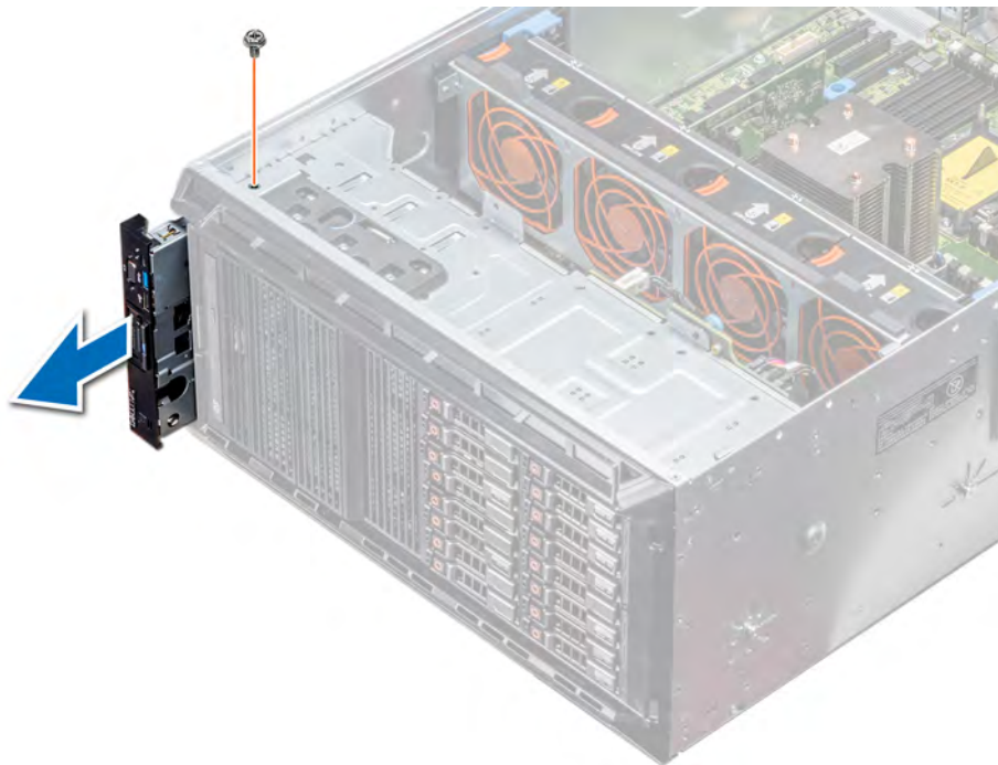
Figure 100. Removing the control panel assembly
