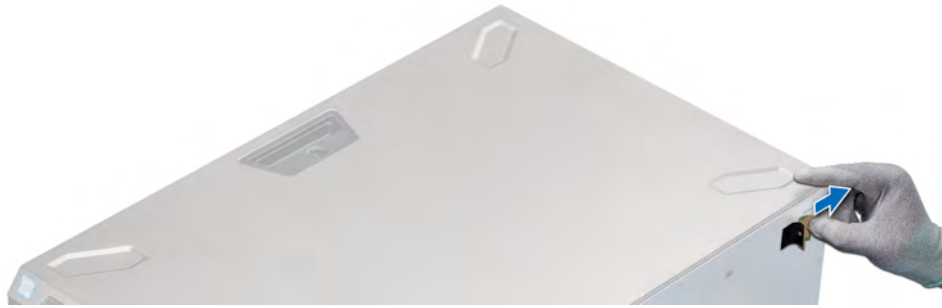
Figure 115. Attaching the mylar cover
