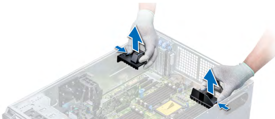
Figure 73. Removing the expansion card holder
