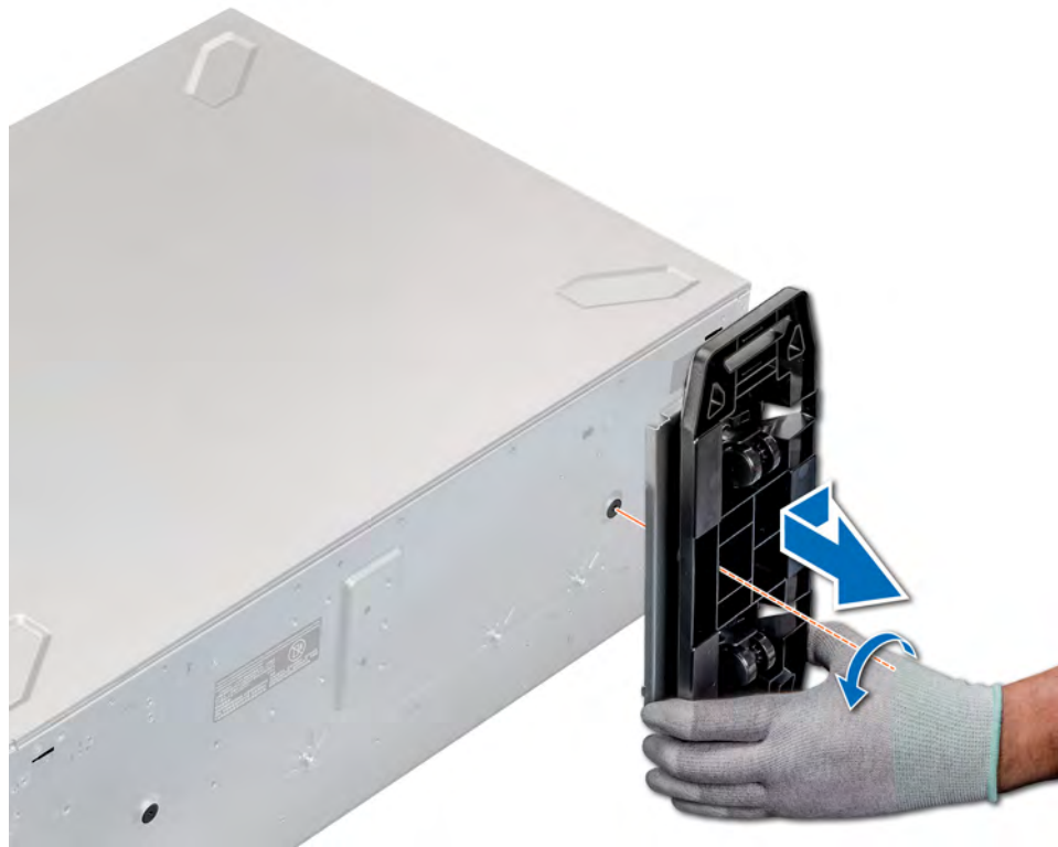
Figure 25. Removing caster wheels
