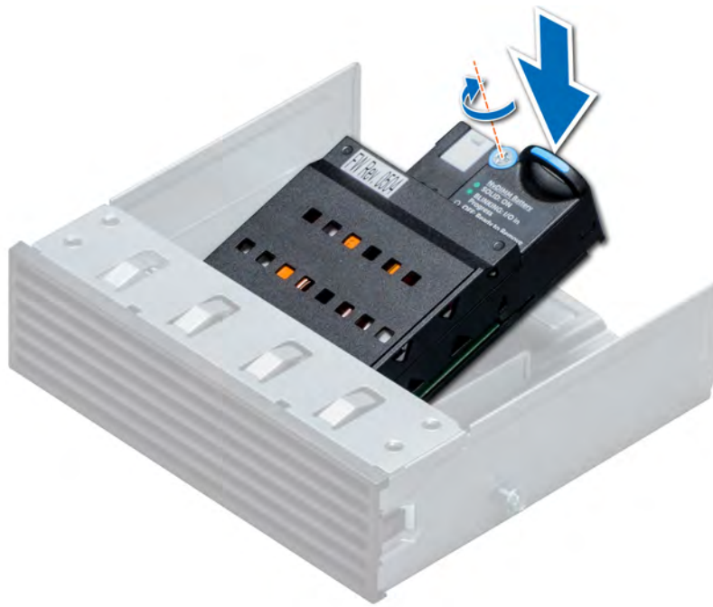
Figure 62. Installing the NVDIMM-N battery
