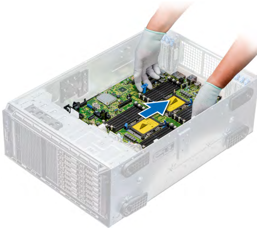
Figure 107. Installing the system board
