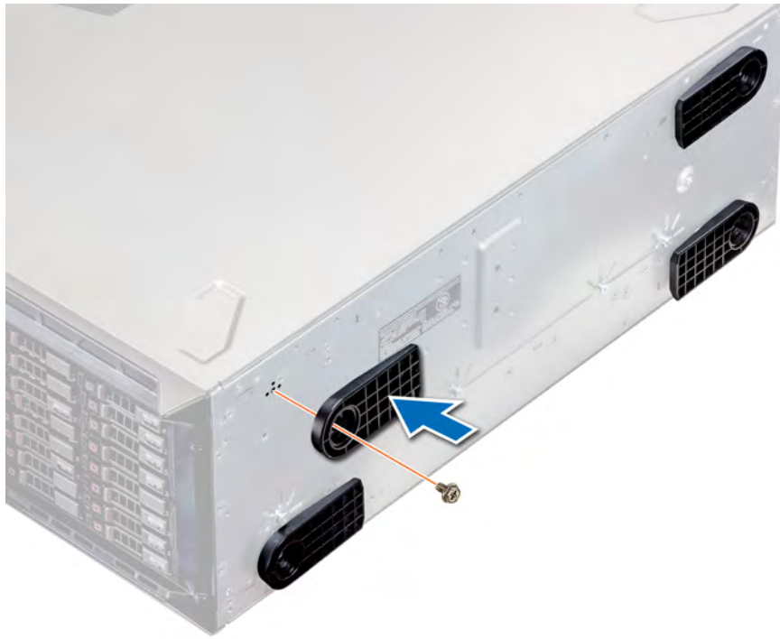
Figure 24. Installing the system feet
