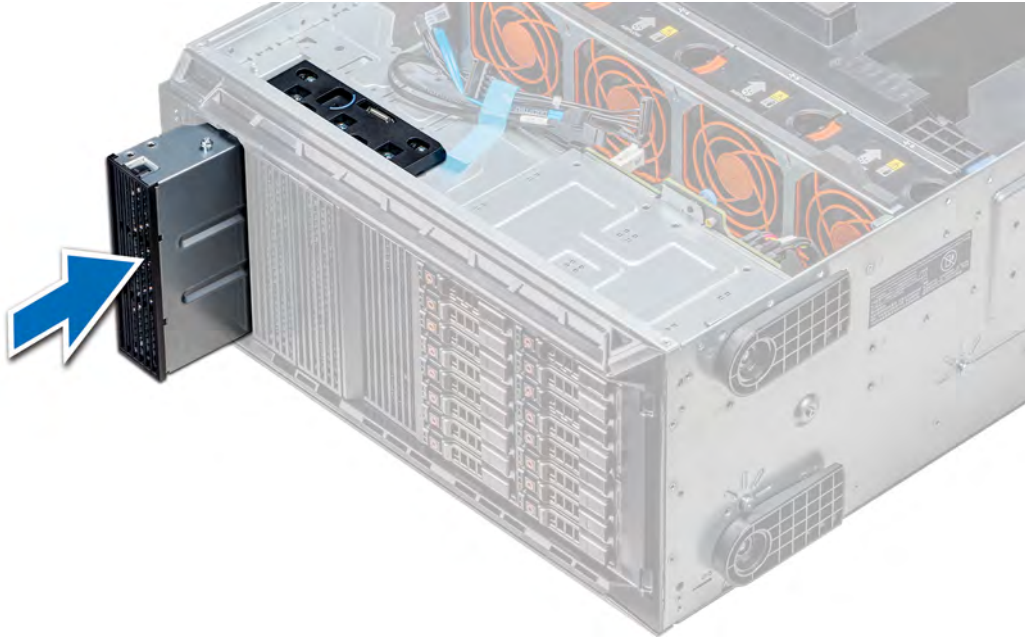
Figure 56. Installing the optical or tape drive blank
