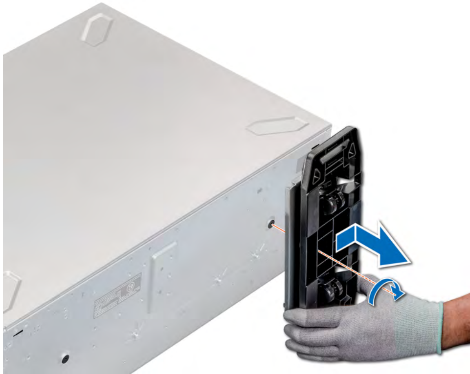
Figure 26. Installing caster wheels
