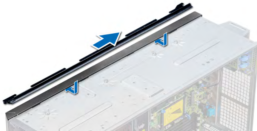
Figure 114. Installing the rack slide cover
