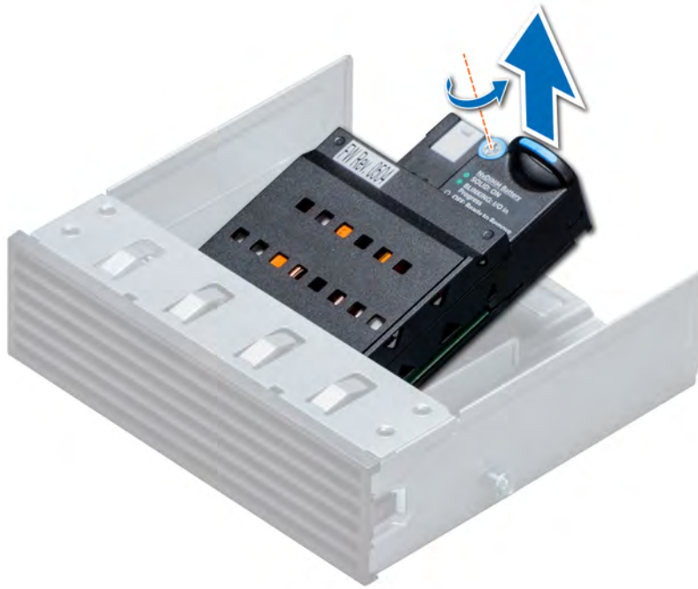
Figure 61. Removing the NVDIMM-N battery
