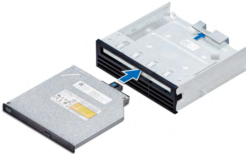
Figure 60. Installing the slim optical drive blank
