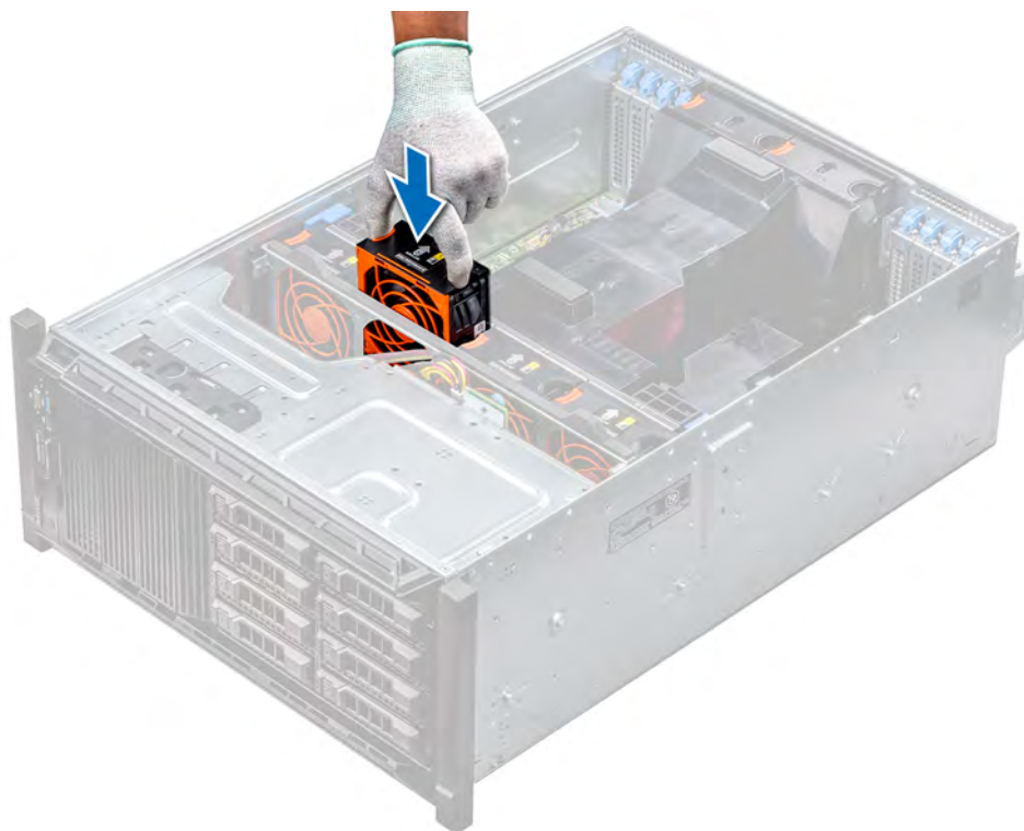
Figure 48. Installing a middle cooling fan
