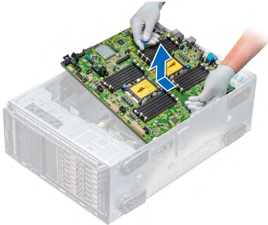
Figure 106. Removing the system board
