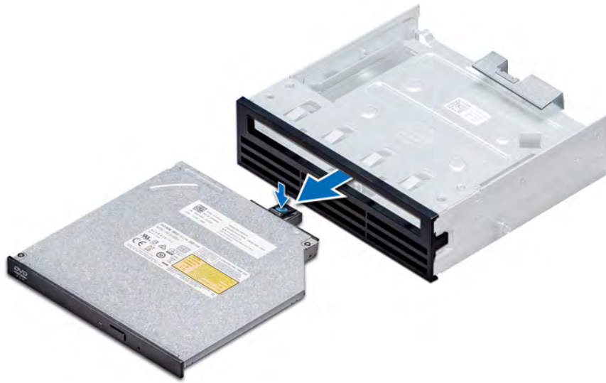
Figure 59. Removing the slim optical drive blank
