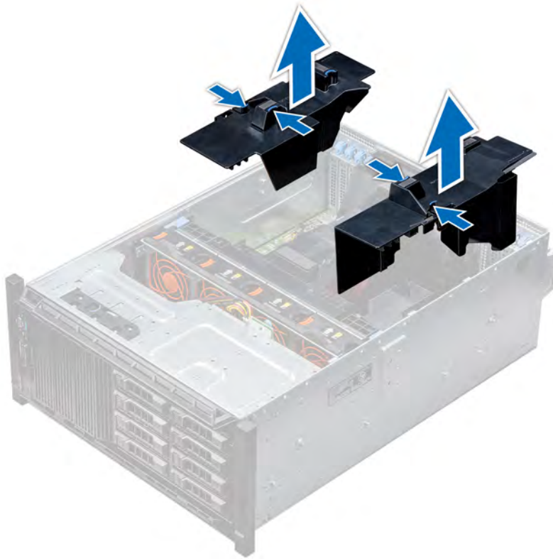
Figure 43. Removing the optional GPU air shrouds
