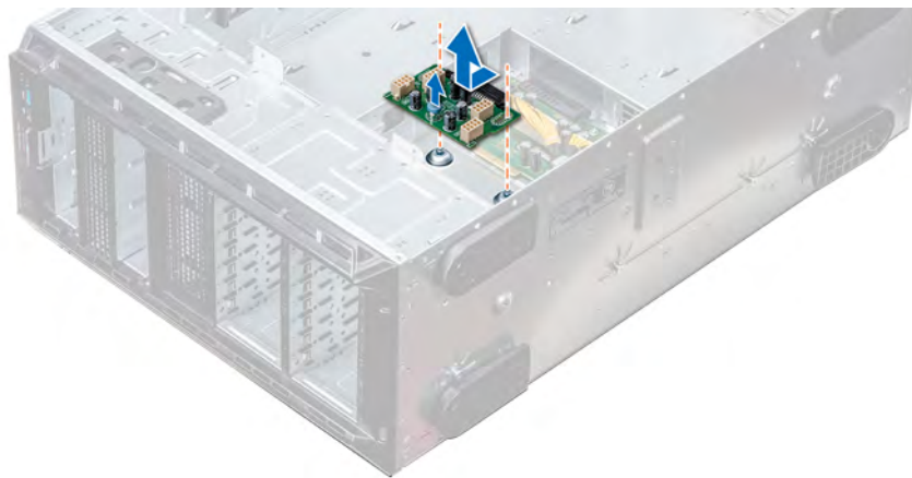
Figure 110. Removing the GPU power interposer board
