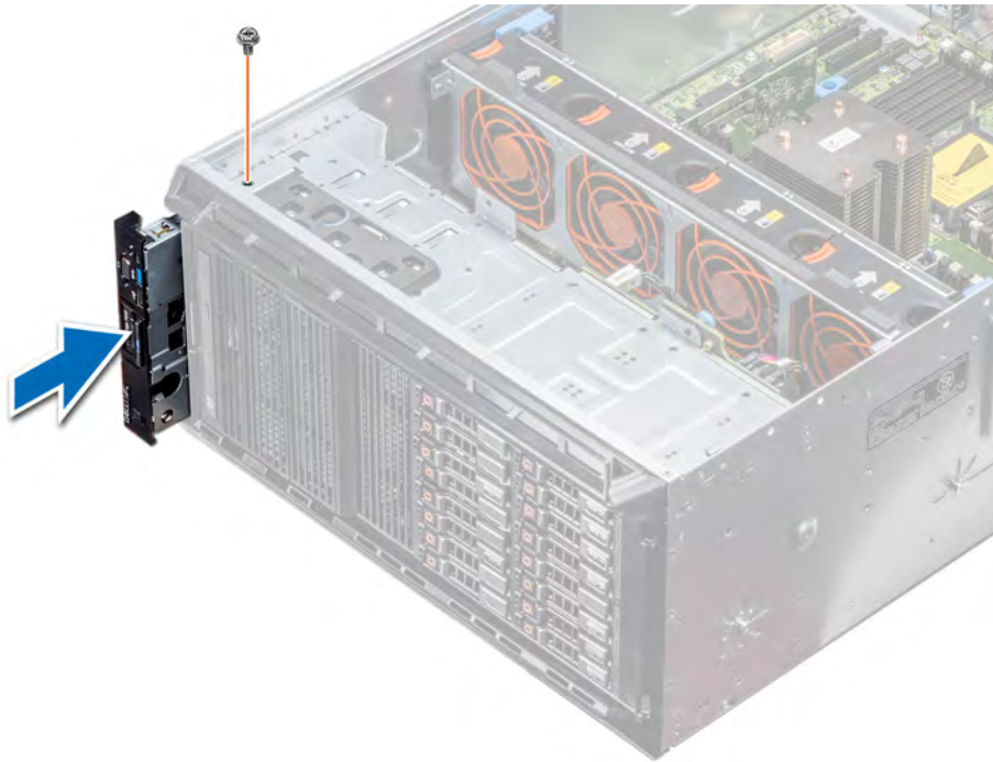
Figure 103. Installing the control panel assembly
