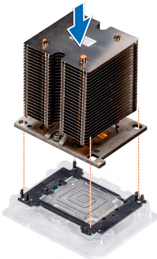
Figure 71. Installing the heat sink onto the processor
