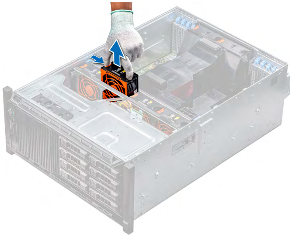
Figure 47. Removing a middle cooling fan
