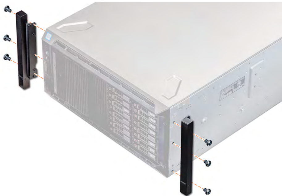
Figure 116. Installing the system ears
