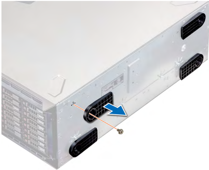
Figure 23. Removing the system feet
