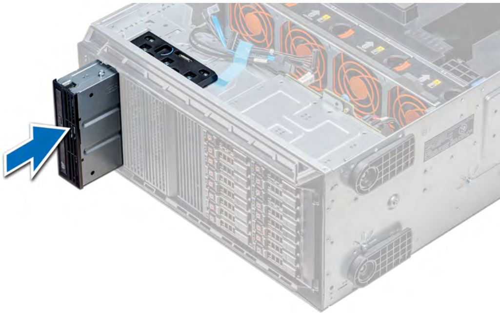
Figure 58. Installing the optical drive cage or tape drive
