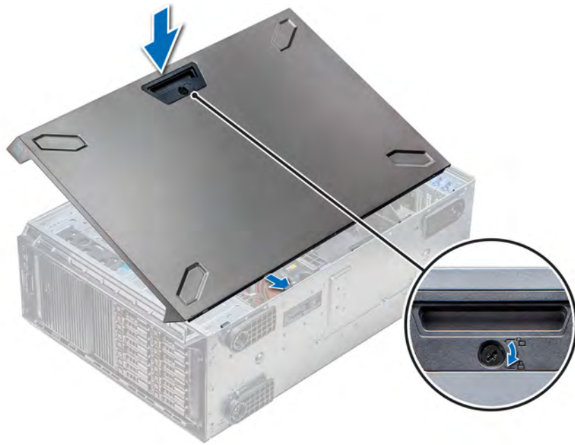
Figure 42. Installing the system cover
