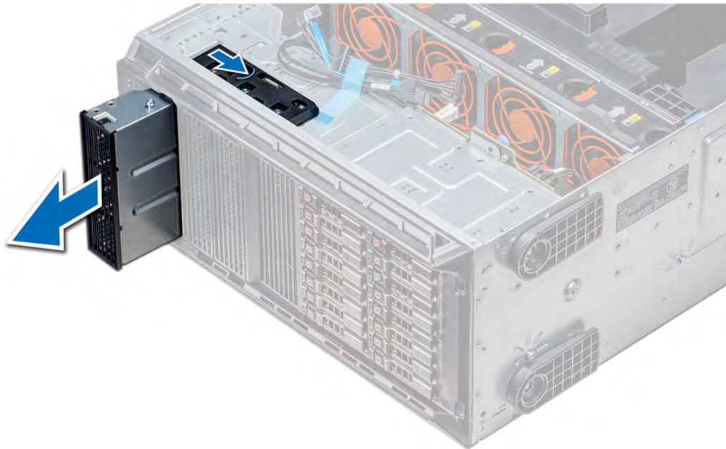
Figure 55. Removing the optical drive or tape drive
