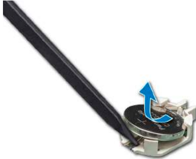
Figure 102. Removing the system battery
