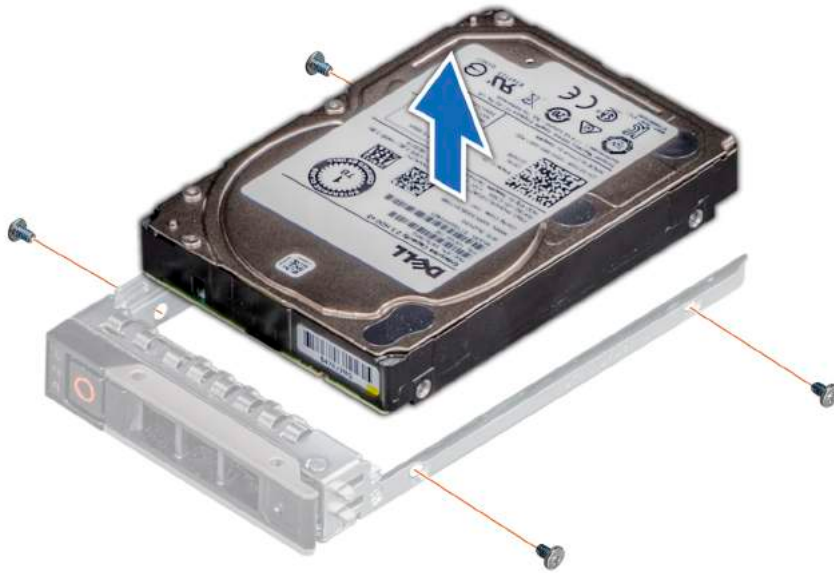
Figure 48. Removing the drive from the drive carrier
