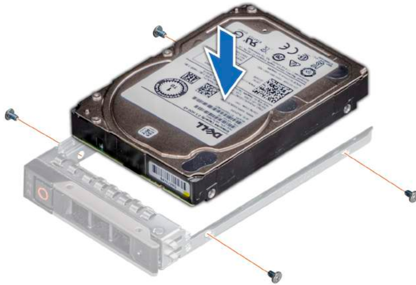
Figure 49. Installing a drive into the drive carrier
