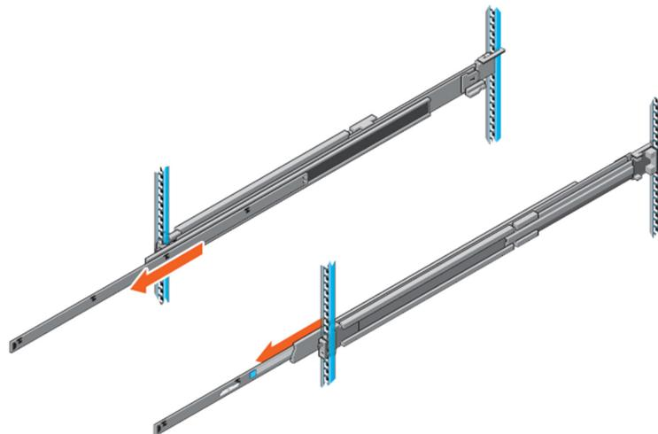
**Figure 37. Pull out inner rail**
