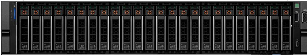
Figure 1. Front view of 24 x 2.5-inch drive system
